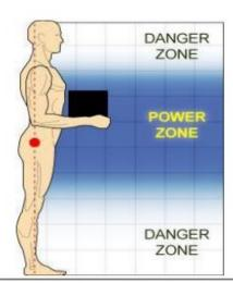
The power zone for lifting is close to the body, between mid-thigh and mid-chest height. Comparable to the strike zone in baseball, this zone is where arms and back can lift the most with the least amount of effort.
